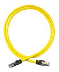
Clarity 6A FTP Modular Patch Cord, yellow, 15', Category 6A, fourpair FTP stranded 26 AWG PVC/CM, center tuned with Clarity 6 A connecting hardware for optimum Category 6A installed performance using Shielded Paralign 2 pair-positioning technology.
