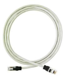
Clarity 6A FTP Modular Patch Cord, gray, 20', Category 6A, four-pair FTP stranded 26 AWG PVC/CM, center tuned with Clarity 6 A connecting hardware for optimum Category 6A installed performance using Shielded Paralign 2 pair-positioning technology.
