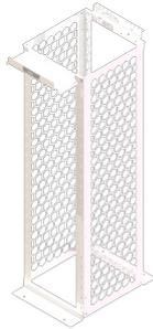
Mighty Mo 20 channel racks are designed to provide greater flexibility and optimum efficiency to any size network. The top trough with built-in waterfall provides bend radius control and efficient patch cable routing. Honeycomb side rails on all depth channel racks provide the ultimate in distribution cable management. The honeycomb side rails, combined with airflow baffles, create a patented system that manages intake and exhaust air from side-vented equipment.
