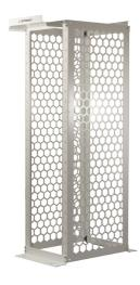
The mighty mo 20 channel racks are designed to provide the greatest in cable management flexibility and efficiency. Honeycomb cutout sidewall allow for infinite cable pathways. The universal 3/8" square hole punch enables mounting of all standard cage nuts and OEM quick mount slides and rails. This creates the industries most versatile equipment rack system.
