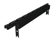
$Mounts \ to \ the \ top \ side \ of \ the \ Mighty \ Mo \ rack \ channels \ or \ frames \ and \ provides \ tool-less \ mounting \ for \ Cablo fill \ cable$ tray to run parallel with the row of racks. Standard brackets position the bottom of the tray at 2" above the rack height and 6" high brackets position the bottom of the tray at 6" above the rack height.
