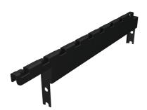
$Mounts\ to\ the\ top\ side\ of\ the\ Mighty\ Mo\ rack\ channels\ or\ frames\ and\ provides\ tool-less\ mounting\ for\ Cablofil\ cable$ tray to run parallel with the row of racks. Standard brackets position the bottom of the tray at 2" above the rack height and 6" high brackets position the bottom of the tray at 6" above the rack height.
