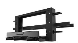
Overhead rack to support additional rack space above existing racks or cabinets. Easily installs to wire cable tray, tubular runway, or threaded rod. The racks are fully assembled and bonded as packaged. The racks are available in 2RU thru 8RU, in black or white to match any installation. Includes a 3 piece waterfall to elegantly route cables down to the lower racks. Used when floor space is at a premium or for easy top of rack cable patching.
