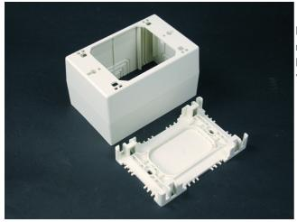
Mounts power/communications devices when additional depth is required. Has combination twistouts for 2700, 2800, 2900 and NM2000 Series Raceways. 4 3/4" L x 3" W x 2 3/4" D (121mm L x 76mm W x 70mm D). 1-Gang.
