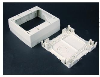
Cover snaps onto base - no screws required. Cover has twistouts on all sides. Rectangular KO in base for extensiion to wall box. Used with 2700, 2800, 2900 and NM2000 Series Raceways. 4 3/4'' L x 4 7/8'' W x 1 3/4'' D (121mm L x 124mm W x 44mm D). 2-Gang.
