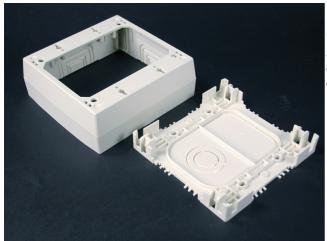
Cover snaps onto base - no screws required. Cover has twistouts on all sides. Rectangular KO in base for extenstion to wall box. Used with 2700, 2800, 2900 and NM2000 Series Raceways. 4 3/4'' L x 4 7/8'' W x 1 3/4" D (121mm L x 124mm W x 44mm D). 2-Gang.
