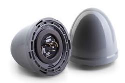
The NWTL-111 BULIT is a distributed-intelligence wireless control node designed to replace standard photocell modules on outdoor lighting fixtures. It connects to a 7-pin twist-lock receptacle compliant with NEMA standard C136.41 to provide ON/OFF and dimming control. The BULIT also connects to a Legrand Wireless Network Manager via a robust and scalable self-healing wireless IP network.
