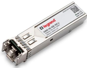
Cisco ONS-SI-GE-SX Compatible 1000Base-SX SFP Transceiver (MMF, 850nm, 550m, LC Duplex, DDM, I-Temp)
