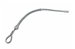
Multi-Weave, Rotating Eye, Cable Diameter - 1.000-1.240-inch, Mesh Length - 52-inch, Eye Diameter - 13/8-inch, Break Strength - 24,600 lbs. Red.
