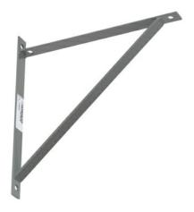
Shelf brackets attach to the wall and extend up to 24 in for heavy duty runway support. Runway is secured to the bracket with J-bolts (included). Made of 3/16 in x 1 in, steel bar. Hardware is zinc plated and dichromated.
