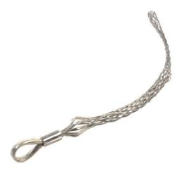
Multi-Weave, Rotating Eye. Cable Diameter - 2.000-2.490-inch, Mesh Length - 50-inch, Eye Diameter - 1 7/8-inch, Break Strength - 48,000 lbs. Yellow.
