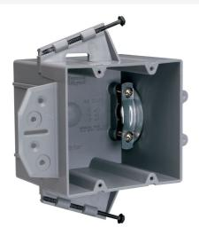
Range or Dryer Box with captive Mounting Screws on Each End. 1/2inch offset for wood or steel stud mounting with metal cable clamp. 12 pack.
