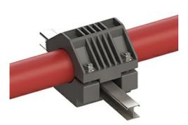
Cablofil cable cleats are designed to restrain cables from lateral and torsional forces supported by ladder tray. In vertical applications, cable cleats provide axial strain relief to cables without damaging the cable sheath. Cablofil heavy-duty cable cleats enclose the cable and the ladder rung with a rigid hi-strength interlocking frame that protects high, medium and low voltage cables from mechanical damage resulting from short circuits.
