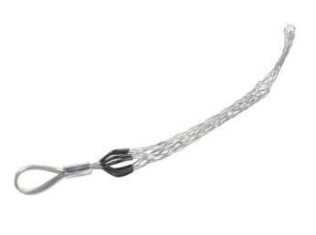
Multi-Weave, Rotating Eye. Cable Diameter - 3.000-3.490"", Mesh Length - 54"", Eye Diameter - 1 7/8"", Break Strength - 48,000 lbs, Aluminum.
