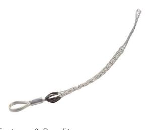
Multi-Weave, Flexible Eye. ◆ Cable Diameter - 3.000-3.490\'\', Mesh Length - 54\'\', Eye Diameter - 5/8\'\', Break Strength - 48,000 lbs.
