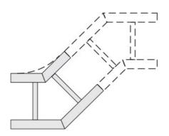
For extremely corrosive applications we offer a full line of straight sections, fittings, covers and mounting accessories in polyester and vinylester fiberglass. Rail heights are available in 4" and 6" and widths are available up to 36".
