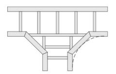
For extremely corrosive applications we offer a full line of straight sections, fittings, covers and mounting accessories in polyester and vinylester fiberglass. Rail heights are available in 4" and 6" and widths are available up to 36".
