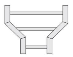
Choose from an extensive selection of metallic ladder tray with a variety of rung and bottom styles to choose from. Finishes include steel, 304L and 316L stainless steel to meet the needs of any application. Rail heights range from  $4""\ \mbox{to }7""\ \mbox{and width sizes are}$ available up to 36"".
