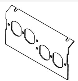
Two (2) duplex KOs. One (1) plate supplied with AC8840 Box. NOTE: AC8840 is a single-service box. Power plates cannot be used in conjunction with communication plates.
