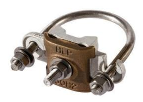
Nominal pipe size range: 3.5" – 4", pipe outside diameter: 3.2" –4.5" Manufactured from electroplated tinned bronze. Conductor range: #6 through 250 MCM PEM stud ensures a flush mounting surface. 5pk.
