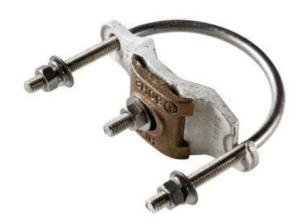
Nominal pipe size range: 3.5" – 4", pipe outside diameter: 3.2" –4.5" Manufactured from electroplated tinned bronze. Conductor range: #6 through 250 MCM PEM stud ensures a flush mounting surface. 5pk.
