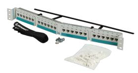
Clarity 6 angled 24-port Category 6 patch panel, high density patch panel is component compliant to TIA/EIA Category 6 performance requirements. White panel occupies 1 rack unit and measures 19"  $\times$  1.75". Jacks are grouped in six-port modules. It is part of the Clarity 6 link and channel solution that provides significant installed performance headroom.
