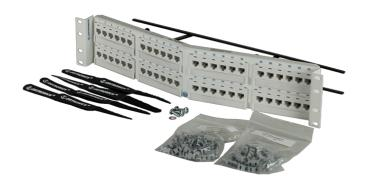
Clarity 6A 48-Port Angled Patch Panel is component compliant to EIA/TIA Category 6a performance requirements. High density white panel occupies 2 rack units, measuring 19" x 3.5". Jacks are grouped in six-port modules. Part of the Clarity 6A link and channel solution that provides significant installed performance headroom.
