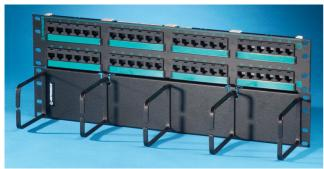
Clarity 5E 48-port high density patch panel with hinged cable management panel is component compliant to TIA/EIA Category 5e performance requirements. It occupies four rack units and measures 19" x 7.0". Jacks are grouped in six-port modules. It is part of the Clarity 5E link and channel solution that provides significant installed performance headroom.
