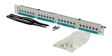
Clarity 6 24-Port high density Category 6 patch panel is component compliant to EIA/TIA Category 6 performance requirements. White panel occupies one rack unit, and measures 19" x 1.75". Jacks are grouped in six-port modules. Part of the Clarity 6 link and channel solution that provides significant installed performance headroom.
