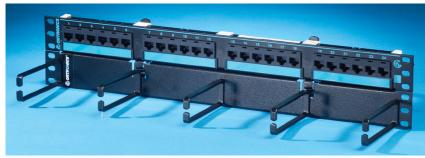
Clarity 6 24-port high density patch panel with hinged cable management panel is component compliant to TIA/EIA Category 6 performance requirements. It occupies two rack units, and measures 19" x 3.5". Jacks are grouped in six-port modules. It is part of the Clarity 6 link and channel solution that provides significant installed performance headroom.
