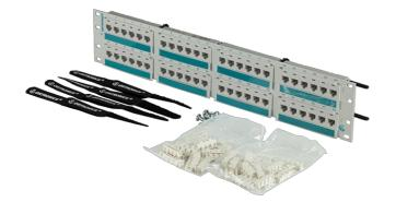
Clarity 6 48-port high density Category 6 patch panel is component compliant to EIA/TIA Category 6 performance requirements. White panel occupies two rack units, and measures 19" x 3.5". Jacks are grouped in sixport modules. Part of the Clarity 6 link and channel solution that provides significant installed performance headroom.
