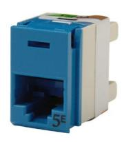
Clarity 5E panel jacks rear load into panels and exceed Category 5e component specifications. Rear load positive latch design, secures mounting of the jack into the panel. Universal T568A/B wiring label and tapered wiring towers simplify termination.
