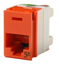
Clarity 5E panel jacks rear load into panels and exceed Category 5e component specifications. Rear load positive latch design, secures mounting of the jack into the panel. Universal T568A/B wiring label and tapered wiring towers simplify termination.
