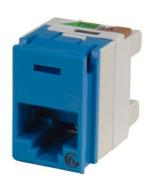
Clarity 6 patch panel jacks, rear load into patch panels and exceed Category 6 component specifications. Rear load positive latch design, secures mounting of the jack into the patch panel. Universal T568A/B wiring label and tapered wiring towers simplify termination.
