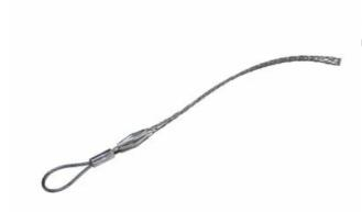
Light Duty, Short Length, ◆ Flexible Eye. ◆ Cable Diameter - 0.500-0.610\'\', Mesh Length - 11\'\', Break Strength - 3,400 lbs.
