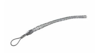
Light Duty, Short Length, ◆ Flexible Eye. ◆ Cable Diameter - 1.750-1.990\'\', Mesh Length - 18\'\', Break Strength - 10,000 lbs.
