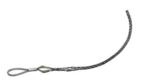
Medium Duty, Flexible Eye. Cable Diameter - 0.370-0.490-inch, Mesh Length - 13-inch , Break Strength - 2,600 lbs.
