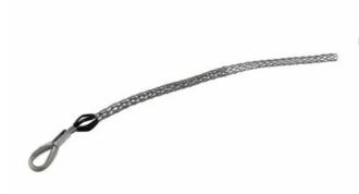
Medium Duty, Short Length, Flexible Eye, T-Type. Cable Diameter - 0.500-0.610-inch, Mesh Length - 21-inch, Eye Diameter - 7/32-inch, Break Strength - 4,500 lbs.
