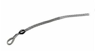
Medium Duty, Short Length, Flexible Eye, T-Type. Cable Diameter -0.500-0.610-inch, Mesh Length - 21-inch, Eye Diameter - 7/32-inch, Break Strength - 4,500 lbs.
