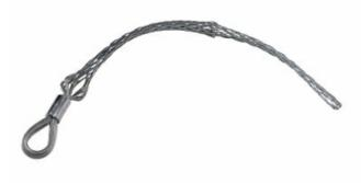
Medium Duty, Short Length, Flexible Eye, T-Type. Cable Diameter - 2.500-2.990-inch, Mesh Length - 24-inch, Eye Diameter - 1/2-inch, Break Strength - 24,500 lbs.
