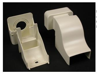
PN5 Series Drop Ceiling Connector for dropping cables from ceiling into the raceway. Has 1/2" and 3/4" concentric trade size KOs. Includes PN153R Reducer Adapter for use with PN03 Series Raceway.
