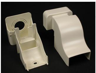
PN5 Series Drop Ceiling Connector for dropping cables from ceiling into the raceway. Has 1/2" and 3/4" concentric trade size KOs. Includes PN153R Reducer Adapter for use with PN03 Series Raceway.
