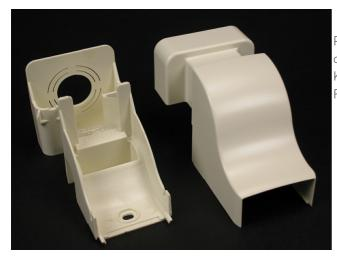
PN10 Series Drop Ceiling Connector for dropping cables from ceiling into the raceway. Has 1/2" and 3/4" concentric trade size KOs. Includes PN153R Reducer Adapter for use with PN03 Series Raceway.
