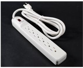
Basic surge protection. Six outlets, lighted switch, impact-resistant putty white polymetric housing, 15A. 6' (1.8m) 14/3 SJT putty white cord with NEMA5-15 plug. Maximum surge current 6500 Amps. 11 3/4"" x 2 1/4"" x 1 1/2 (298mm x 57mm x 38mm). Keyhole mounting.
