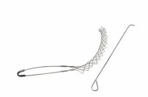
Heavy-Duty, Short Length, Rotating Eye, K-Type. Cable Diameter - 1.500-1.990-inch, Mesh Length - 25-inch, Eye Diameter - 1 5/8-inch, 27,200 lbs.
