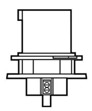
Triple-Pole, 4-Wire, Pin and Sleeve Inlet. 20A, 3/250V.
