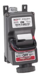
Triple-Pole, 4-Wire, Non-Fusible Mechanical Interlock Receptacle. 20A, 3, 240V.
