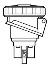
Pin and Sleeve3 pole 4-Wire 30A 3-Phase 480V Receptacle
