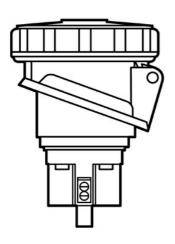
4-Pole, 5-Wire, Pin and Sleeve Receptacle. 100A, 3Y, 347/600V.
