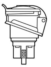
Splashproof Receptacle, 4 Pole 5 Wire, 63A IP44 Suitability. 200/346, 240/415V
